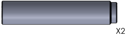
5: LONG CYLINDER SPACER (3.625 INCHES)
