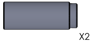
7: SHORT CYLINDER SPACER (2.00 INCHES)
